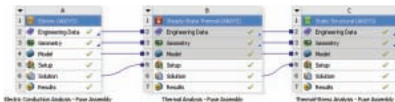
The project schematic shows the multiphysics workflow for a coupled electric conduction, heat transfer and subsequent thermal stress analysis.
