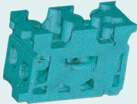
This detailed finite element model contains more than 26,000 solid elements to accurately represent the intricacies of the Mazzucconi engine block casting.
