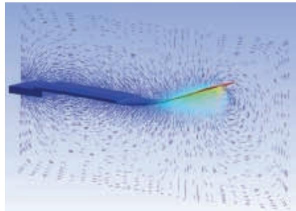
ANSYS Multiphysics software was used in optimizing a piezoelectric fan blade geometry to produce a resonant frequency exactly at 60 Hz and in evaluating the motion of the fan blade and resulting air flow.
