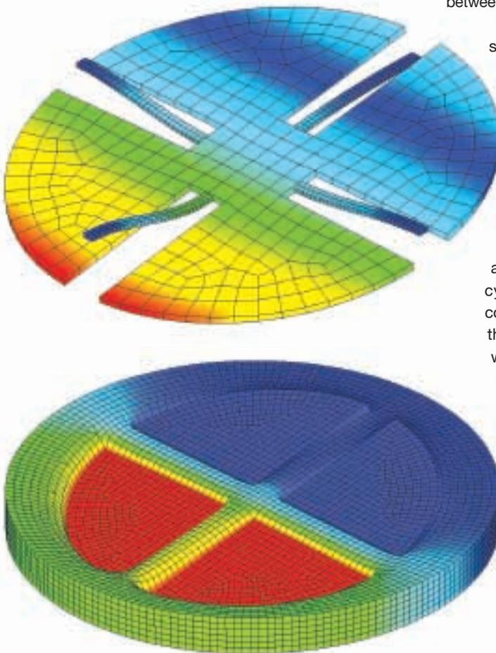
The switching speed and positioning of a MEMS digital micromirror was studied by sequentially coupling the analysis of models for structural deformation (top) and electrostatics (bottom).
