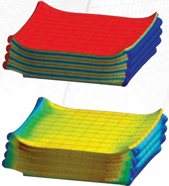
Electric potential (top) and equivalent stress (bottom) simulation results for a folded dielectric elastomer actuator
