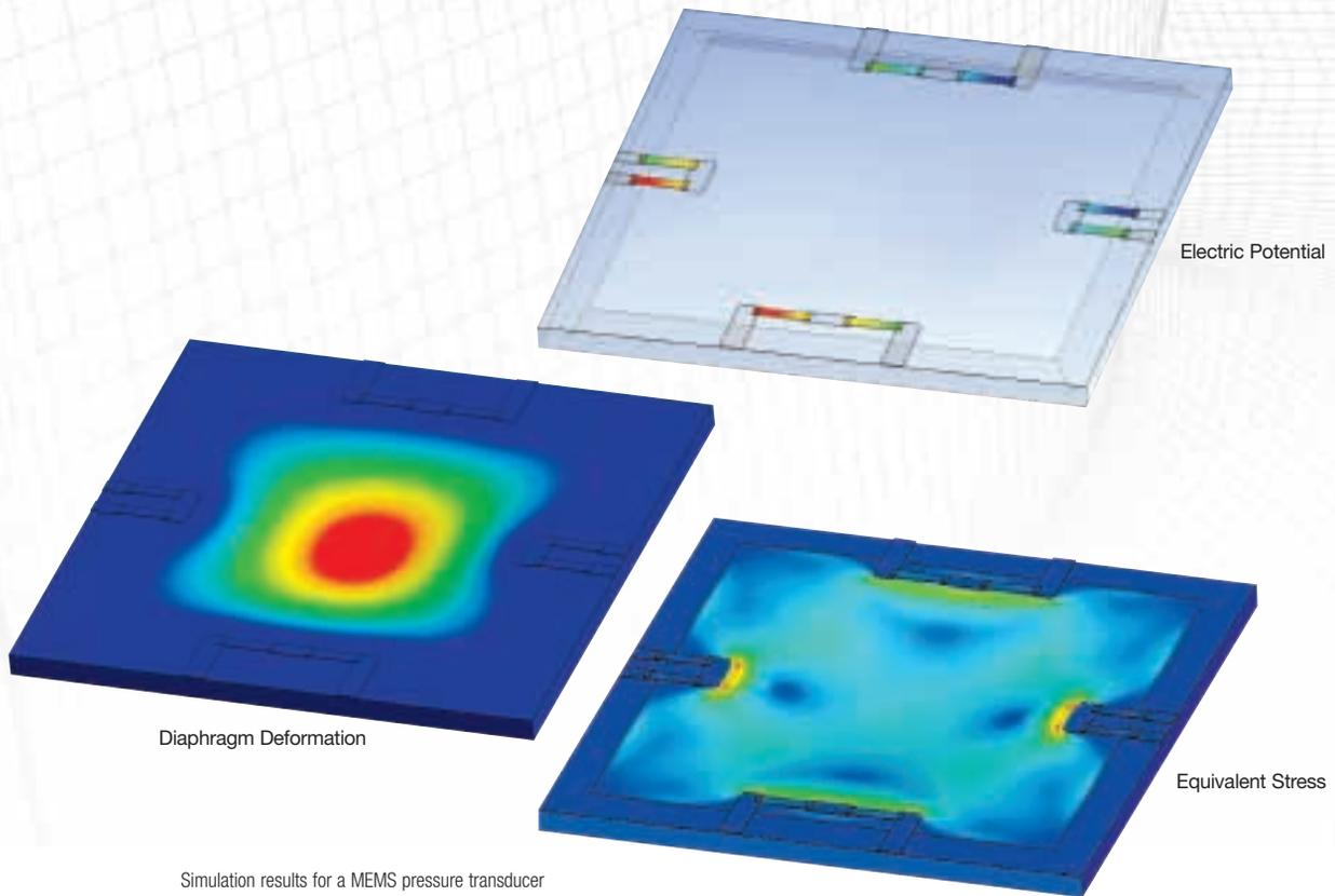
Simulation results for a MEMS pressure transducer
