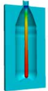
Polyflow makes it possible to study the behavior of plastics and other materials, such as this example of injection stretch blow modeling using shell elements. The image shows thickness distribution.
