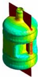
Simulation helps companies to reduce product failure risk early in the design cycle by providing insight into critical parameters/characteristics, such as material distribution (left) and top load stress distribution (middle) in a five-gallon blow-molded water cooler bottle (right).
