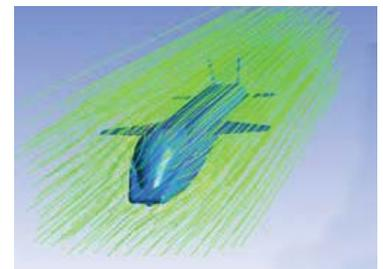
ANSYS CFX helped develop the overall streamlined shape of the external fairing
