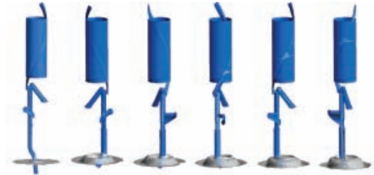
Evolution of the free surface of oil in a reciprocating compressor. The blue area is the gas/oil rotating domain inside the shaft, and the gray surface at the bottom shows the oil level of the reservoir. As the shaft rotates, oil is pumped up due to body forces. Image courtesy Embraco.
